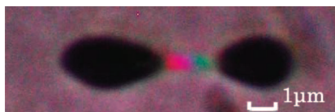
Figure 4. An optical micrograph of hollow channel exposed
